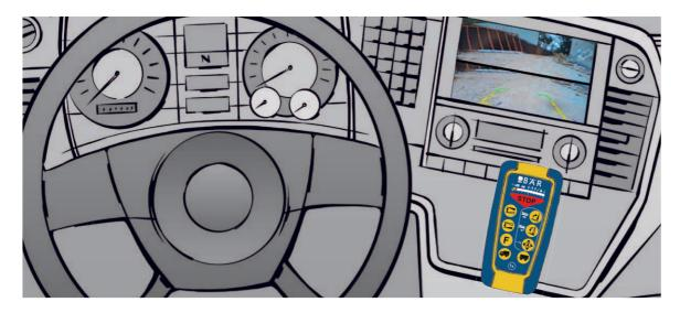
Manoeuvring with the truck and Standard Cargolift at the ramp requires extensive practice — or the Bär SmartControl CabinControl. Together with two rear drive cameras and a monitor in the cabin, you can operate and bring the Cargolift perfectly into position — if desired with orientation lines on the monitor (patented).
